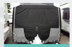
On a number of Coachman caravans there is an additional fixing point. The large flap located at the top of the cover hooks over the Coachman sign located above the front window. Please see image of how the cover should be fitted This is not standard on all Coachman covers. If you are unsure of how this section is fitted please contact our customer service team.
